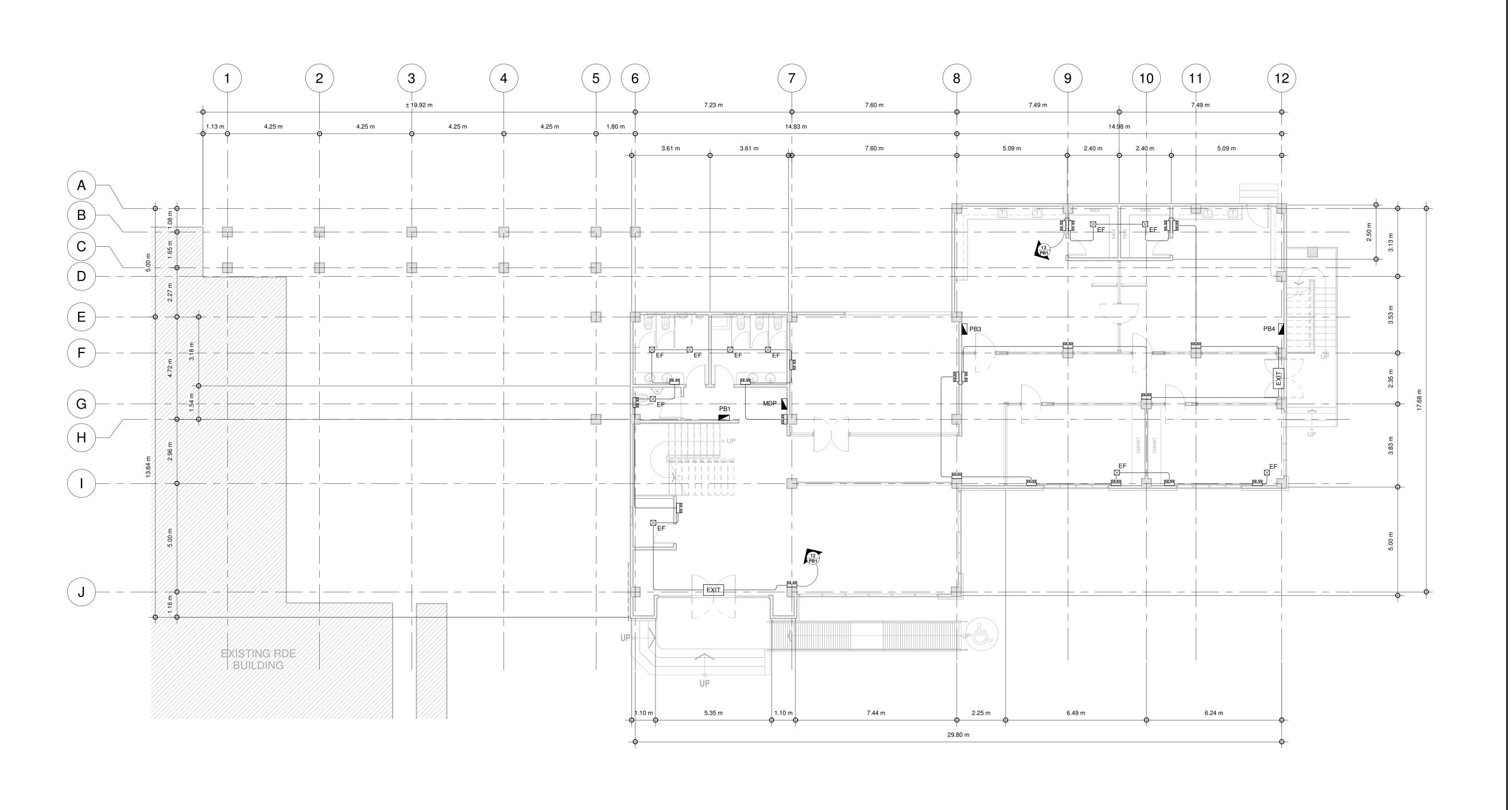
GROUND FLOOR EXHAUST FAN, EMERGENCY LIGHT & EXIT SIGNAGE LAYOUT PLAN
